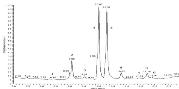
Figure 3. Ion chromatogram of (1) nornordihydrocapsaicin, (2) nordihydro-capsaicin, (3) N-vanillyl-nonanamide, (4) capsaicin, (5) dihydrocapsaicin, (6) N-vanillyl-decanamide, (7) homocapsaicin, (8) homo-dihydrocapsaicin isomer I and (9) homodihydrocapsaicin isomer II in "Superhot" chilli sample (S4)
